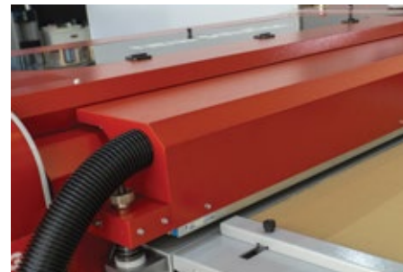
• Self-cleaning system - system composed by an ionizing bar and a vacuum.
